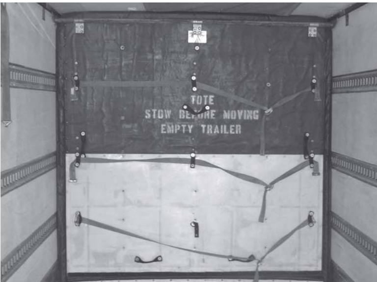
6. Load securing strap and E track latched, but not pulled tight, unsafe.
