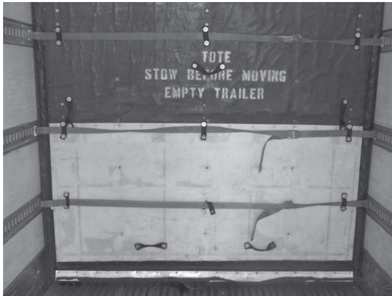
7. Load securing straps properly applied.
